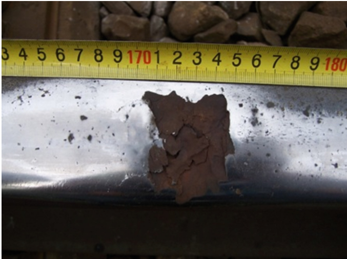
Fig. 6. Defect with a short length and a significant width (the difference between defect length and its diameter \delta(A) )
