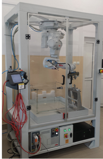
Fig. 7. Robot-assisted vane thickness measurement stand.
