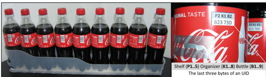
Fig. 4. Selected organizer with electronically marked bottles
