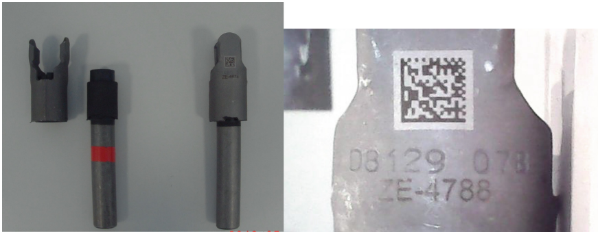
Fig. 5. Car steering column couplers, left – item after test, dissection – negative result of test. Right – correct item with burned individual pictogram (QR code).
