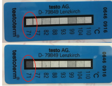
Fig. 16. Temperature indication before (up) and after (down) temperature test cycle
