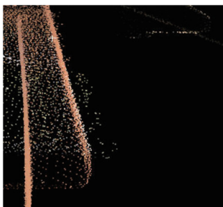
Fig. 8. An example of a blurring cloud of points on a shiny glossy kitchen countertop.
