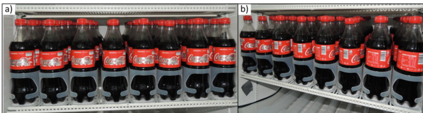
Fig. 12. Electronically marked bottles with transponders directed towards: (a) door, (b) side walls of the refrigerator
