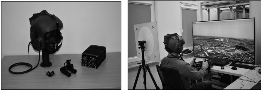
Fig. 2. View of the NSC-1 Orion helmet-mounted cueing system (left side) and the magnetic field generation system with the flat coil at the flight simulator station (right side) [15]
