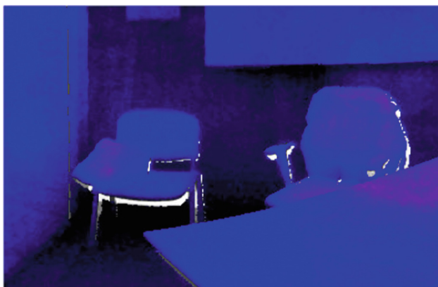
Fig. 1. A combination of two armchairs - an employee sat on the right armchair before scanning. It is in parts adjacent to the body about 1 °C warmer.
