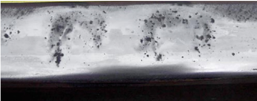
Fig. 2. Typical forms of squat-type defects: V-shaped crack (left) and arc-shaped crack (right).
