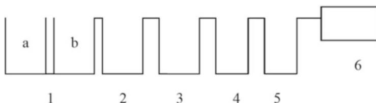
Fig. 3 Schematics of the various basins of the Skikda refinery effluent treatment unit. Basin 1 (a) and (b) are used for the screening of big chunks; basin 2 is primarily for decantation and scraping off of the precipitated elements; basin 3 is used for the flocculation of the effluents; basin 4 is the microbiological basin where the biodegradation of the effluents starts using microorganisms solutions, aided with proper oxygenation and clean water source; basin 5 is a secondary decantation basin; and finally basin 6 is a sand filter
