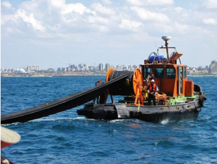
Fig. 17 An exercise in Ashkelon Port, deploying a sea boom. Source: MEPD, Israel
