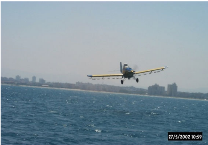
Fig. 18 An exercise in Haifa bay, dispersing oil with spraying aircraft, 2002. Source: MEPD, Israel
