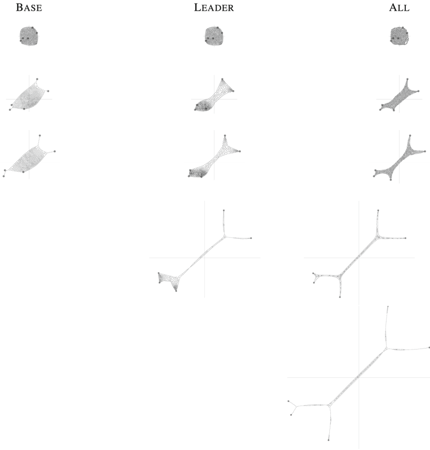
Fig. 12. A comparison of strategies for the same example, for a swarm with n = 400 and failure rate 0. As indicated, columns correspond to strategies BASE, LEADER, and ALL. Rows show the swarms at times T = 200 , T = 2000 , T = 3000 , T = 7600 , T = 12,000 , with 60 steps per simulated second. When a swarm is no longer shown, it has become disconnected right after the previous time step.
