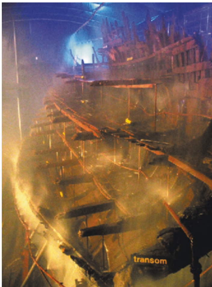
Fig. 3.1 The sixteenth century warship Mary Rose undergoing spray treatment with solutions of PEG200 and PEG2000 at HM Naval Base dry-dock in Portsmouth, UK. (Image reproduced with permission from the Mary Rose Trust)
