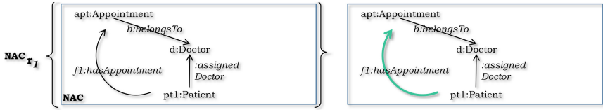
Fig. 3. Transformation rule r_1 for individual resource allocation of patients. (Color figure online)
