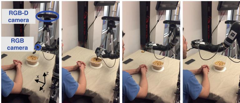
**Fig. 1.** Our feeding system includes a MICO robot arm, an RGB-D camera, and an RGB camera. The first image also labels the axis orientations of the robot coordinate system. (Color figure online)
