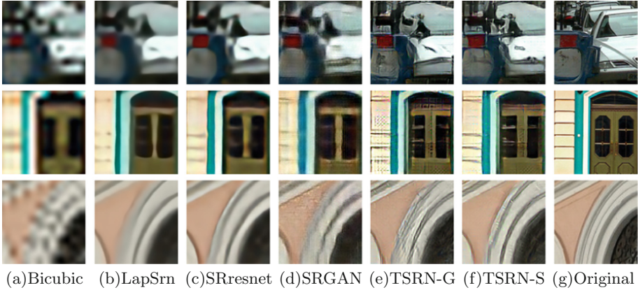
Fig. 6. Visual comparison of recent state-of-the-art methods based on distortion metrics and perceptual quality with our texture based 8\times image super-resolution.
