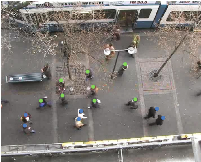
Fig. 1. Each pedestrian is represented by a single keypoint. Pedestrians walking in the same direction are clustered into one group s_i . In this example, two sets of pedestrians going in opposite directions are identified.
