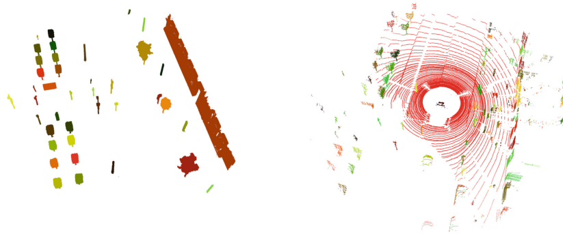
(a) Landmark objects of the HD map (b) Detected objects in RMB Lidar frame
