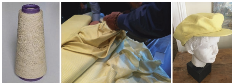
Fig. 9 Yarns, fabrics and garments obtained from processing GINEXTRA® fibres in industrial plants
