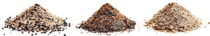
Fig. 1 (Left) Mix 1—palm kernel shells and rice husks, 50/50 w/w. (Center) Mix 2—palm kernel shells and animal meat and bone meal C1, 50/50 w/w. (Right) Mix 3—rice husks and animal meat and bone meal C1, 50/50 w/w. All weights on as-received basis
