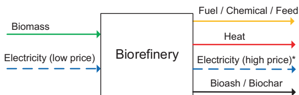
Fig. 10 Diagram of a biorefinery based on gasification or pyrolysis integrated with water/steam electrolysis. (Asterisk) The electricity output can be produced by a heat engine or by a reversible electrolysis system (e.g., solid oxide cells)
