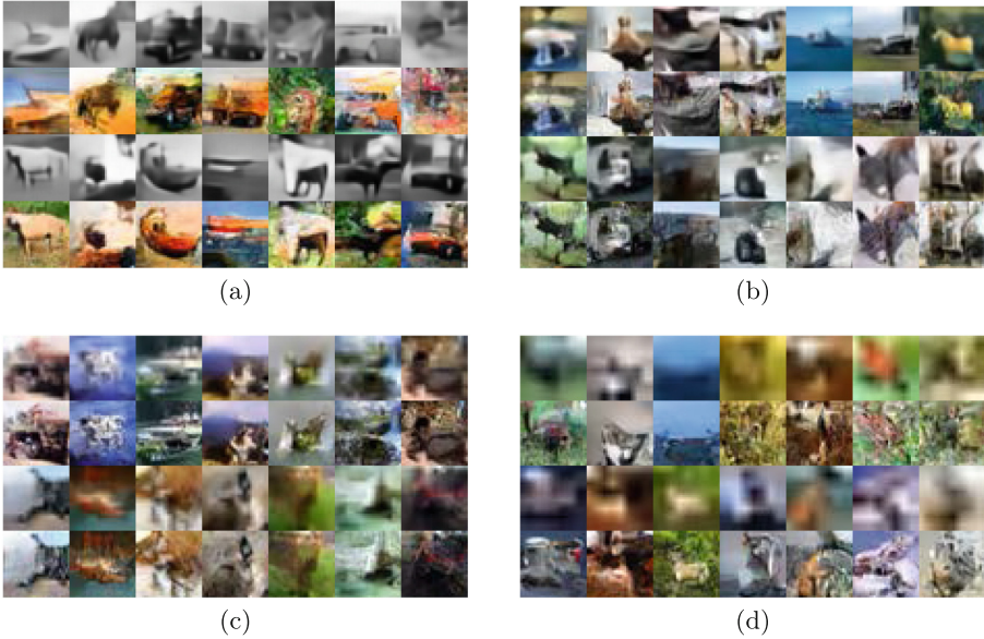
Fig. 9. Samples from models trained with grayscale auxiliary images with 16 color levels (a), 32 \times 32 auxiliary images with 32 color levels (b), and at reduced resolutions of 16 \times 16 (c) and 8 \times 8 pixels (d) with 256 color levels. For each model the auxiliary representation f(\mathbf{z}) , with \mathbf{z} sampled from the prior, is displayed above the corresponding conditional pixelCNN sample. (Color figure online)
