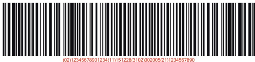
Fig. 11.1 GS1-128 Barcode used in the meat industry
