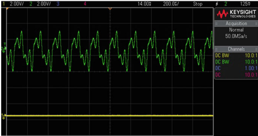
Fig. 16.6. Time domain oscilloscope image of 0-0-0 where green is the oscillator’s output and yellow is the microcontroller’s logic level
