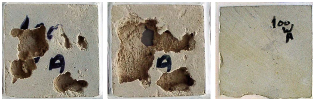
Fig. 12 Erosion characteristics of Wacker-OH-treated Mokattam samples after (CHL) artificial aging
