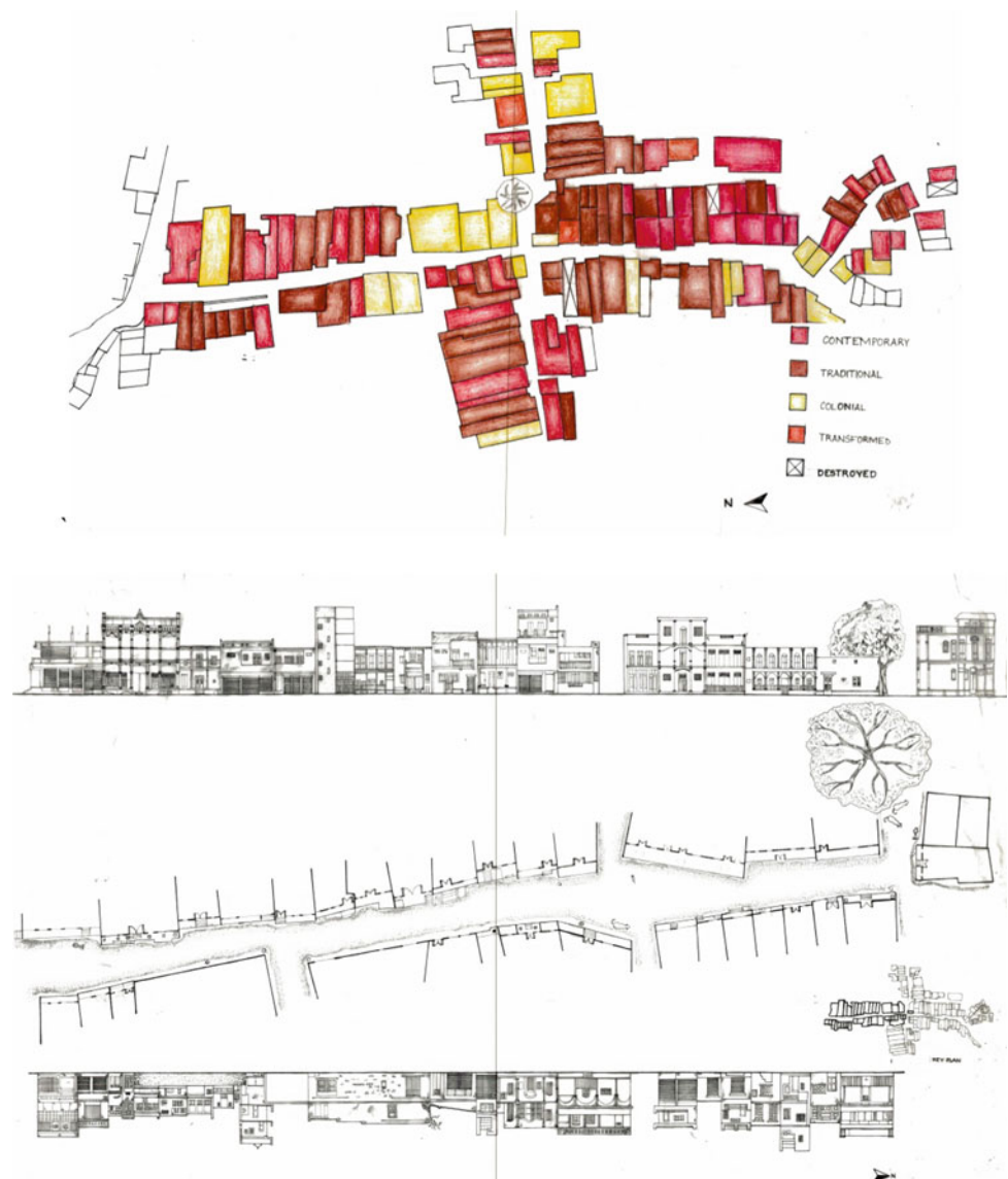
Fig. 4 Transformation of built from traditional to contemporary evident in the street plans above and elevations below at Patan. Source Documentation of Patan, design studio first year (2013–14), studio co-ordinator; author, University School of Architecture and Planning, GGSIPU, Delhi, India
