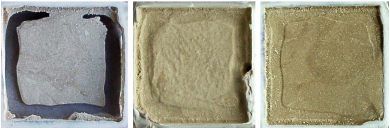
Fig. 6 Erosion characteristics of B-72-treated Tura-Ma'sara limestone samples after (CHL) artificial aging
