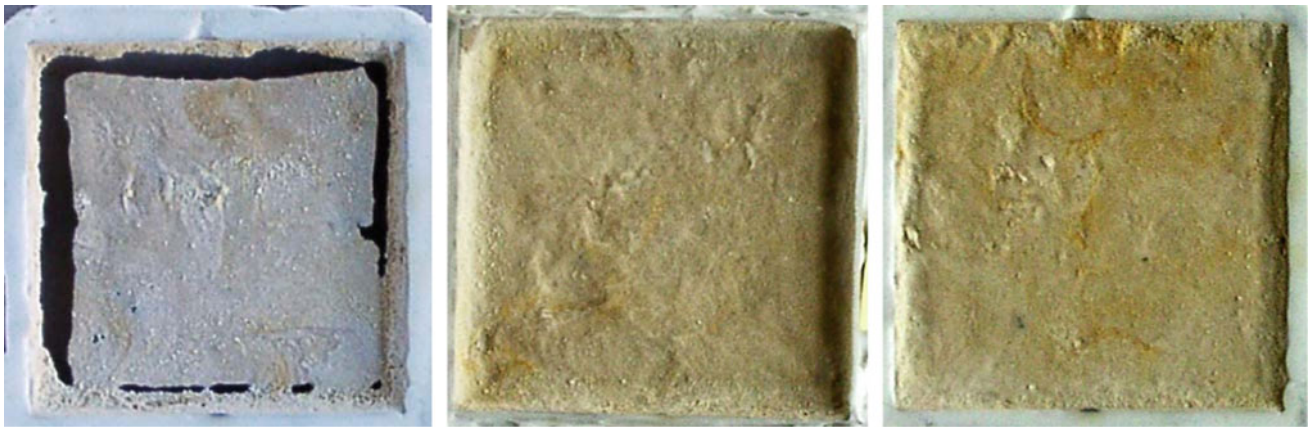
Fig. 7 Erosion characteristics of Wacker-OH-treated Tura-Ma'sara samples after (CHL) artificial aging
