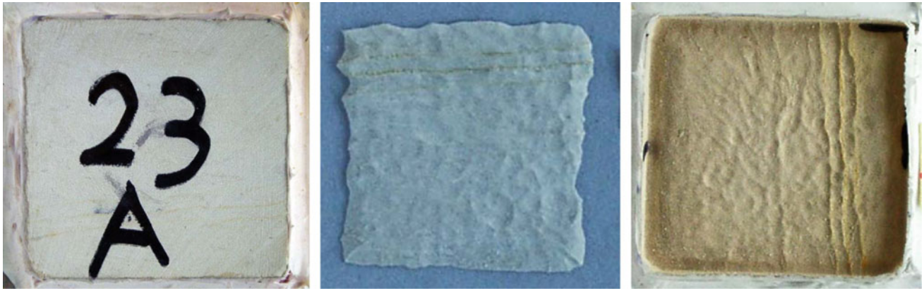
Fig. 4 Erosion characteristics of untreated Tura-Ma'sara limestone samples after (CHL) artificial aging
