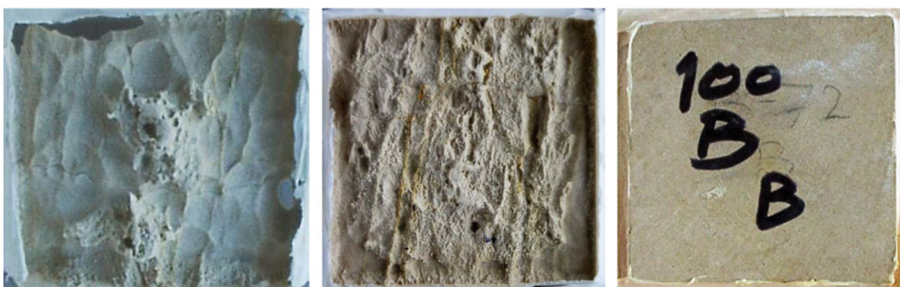
Fig. 11 Erosion characteristics of B-72-treated Mokattam limestone samples after (CHL) artificial aging
