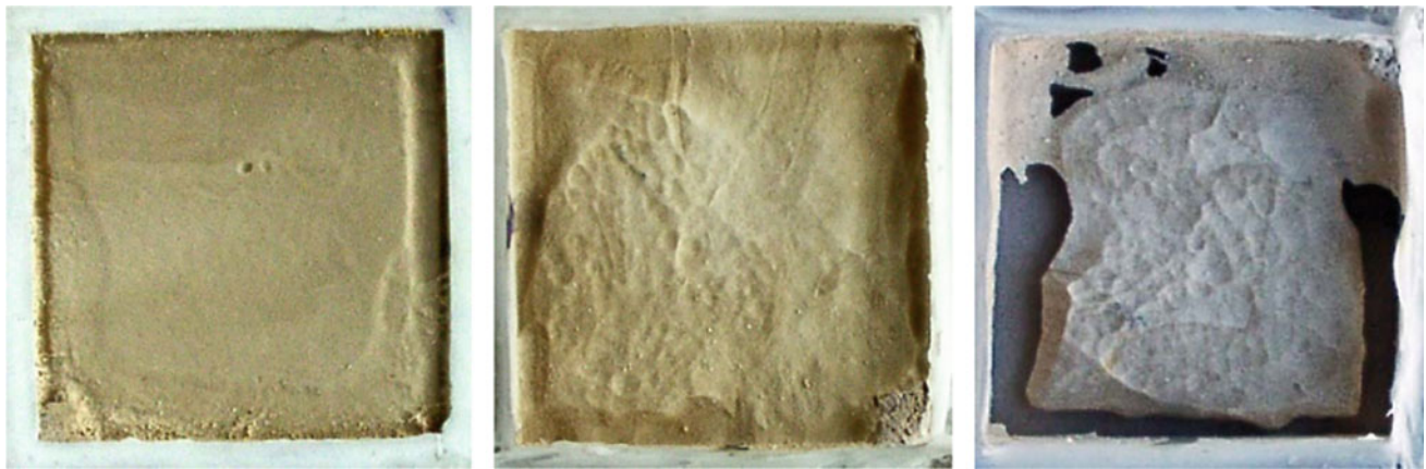
Fig. 5 Erosion characteristics of acrylate-treated Tura-Ma'sara samples after (CHL) artificial aging
