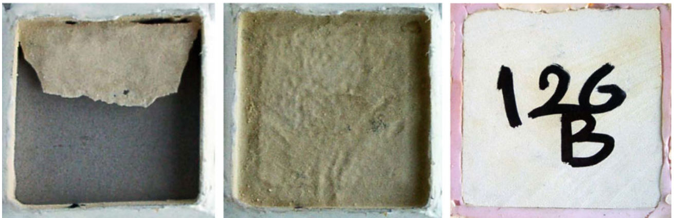
Fig. 9 Erosion characteristics of untreated Mokattam limestone samples after (CHL) artificial aging
