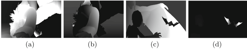
Fig. 1. Two sample optical flows extracted from the Sintel database. Horizontal components in (a) and (c); vertical components in (b) and (d). White corresponds to flow in the positive direction (right or up) and black corresponds to the negative direction.
