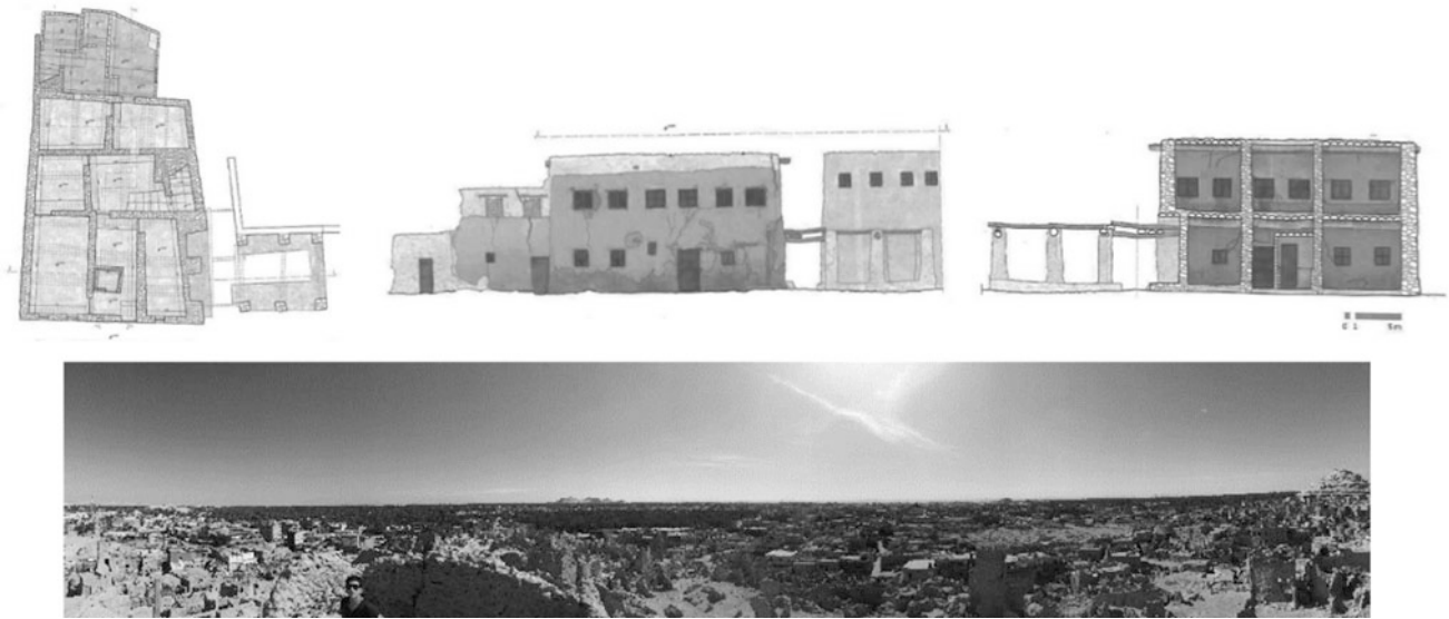
Fig. 9 Plan, front view, and section of the survey of a house in Shali, Siwa Oasis (Oasi Di Siwa book) and a panoramic photograph by the author
