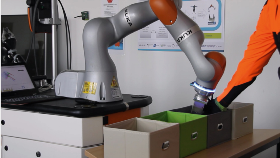
Fig. 2. Robotic co-working in the Cinderella case study. Every box has an associated autonomous controller watching safety of encounters of a human with robot. Box 1 is on the left, box 4 on the right.
