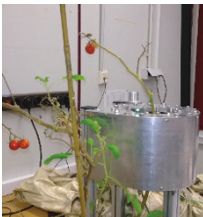
Cherry tomato plant in a center-field Halbach magnet
