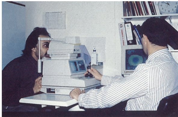
Fig. 2.4 Videokeratoscope. The patient places his or her chin and forehead on the rest and fixates the central target, whilst the operator aligns the machine with the corneal reflex
