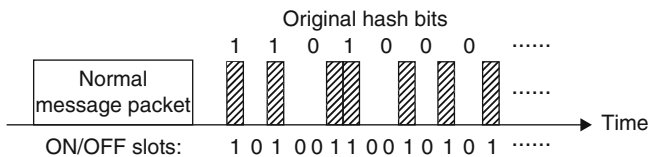
Fig. 5.1 The messaging structure of message integrity protection and authentication
