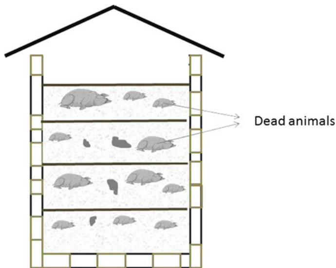
Fig. 5.6 Schematic of conventional composting system for dead animals
