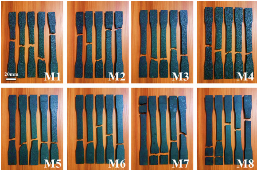
Fig. 6 Fracture of specimens after tensile stress
