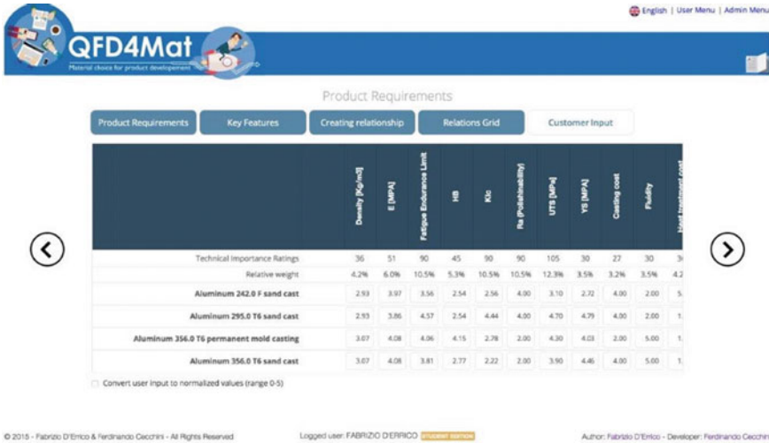
Fig. 3 Example of calculation box for the assessment of key features and the relative weighted score for competing products in a classroom case studied regarding with new lightweight automotive suspension arm. The screenshot is provided by the commercial edition of the tool
