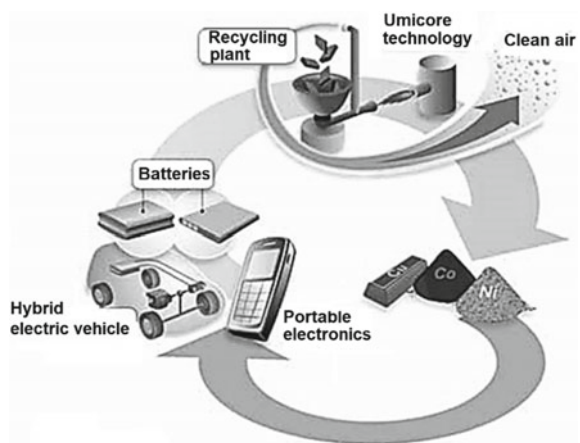
Fig. 1 Schematic diagram showing the recycling of batteries at Umicore with a closed loop of metals. Modified from [1]
