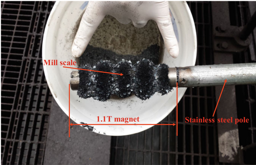
Fig. 4 Mill scale recovered by the 1.1T magnet separator mounted on a stainless steel pole
