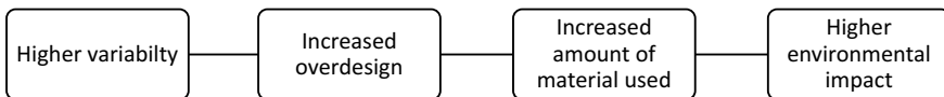
Fig. 2 A schematic of the connections between manufacturing variability and environmental impact. If the variability of a process is high, then there is a need for overdesign to account for this additional variability. More material is needed to satisfy these additional design requirements, which leads to more environmental impact
