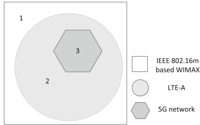
Fig. 1. The 5G heterogeneous wireless network system.
