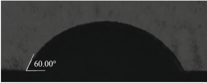
Fig. 3 Contact angle of sample 2 tested by the sessile drop method
