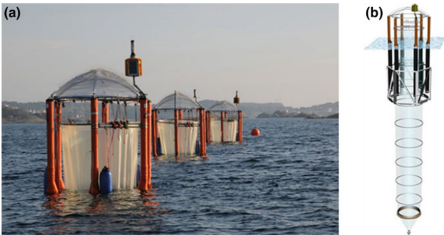
Fig. 2 a A series of Kiel Off-Shore Mesocosms for Ocean Simulations (KOSMOS) in the Northern Baltic Sea. The mesocosms were successfully employed in long-term experiments in different climate zones, from the high Arctic to the subtropics. Experimental perturbations include the addition of inorganic nutrients or organic compounds, \text{CO}_2 enrichment, manipulation of mixed layer depth, simulation of deep-water upwelling, species exclusion and addition of invasive species. b A mesocosm, consisting of a floatation frame and a flexible bag 2 m in diameter and 20 m in length. After deployment, the bag unfolds by weights pulling down its lower end to depth, thereby enclosing an undisturbed water column 55 \text{ m}^3 . The bag is then closed at the bottom by a full-diameter sediment trap (Riebesell et al. (2013). https://www.geomar.de/en/research/fb2/fb2-bi/infrastructure/kosmos-kiel-off-shore-mesocosms-for-oceanographic-studies ). With permission by Gerd Hoffmann-Wieck
