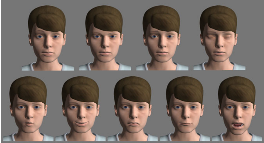
Fig. 8.3 Blend shapes used in our pipeline. From left to right and from top to bottom: eyebrows up (AU2), eyebrows down (AU4), inner eyebrows up (AU1), eyelids down (AU43); lips funneled (AU22), smile (AU12), lip corners down (AU15), lips pressed (AU24) and mouth open (AU27)
