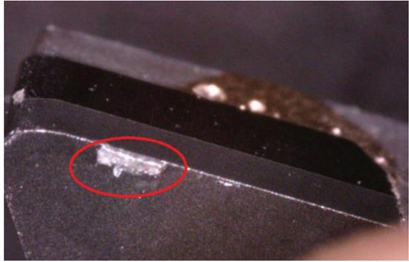
**Fig. 14** Failed part which is causing the change of 3. PCD tool. Intermetallic can be seen clearly
