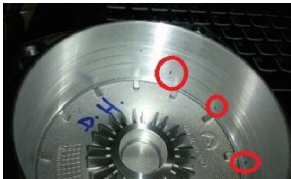
**Fig. 13** 3. PCD tool is in 95th part. As seen is the damaged area is clearly broken and it is not shear plane area; it's on rake angle area
