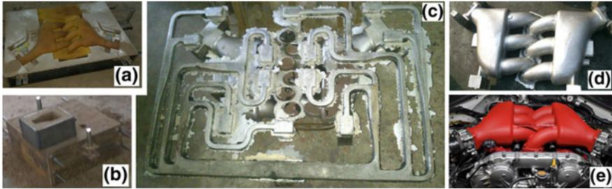
**Fig. 10** Filter casting pictures: **a** the green sand mold and cores **b** the assembly **c** the bottom view of the casting **d** the top view and **e** the mounting
