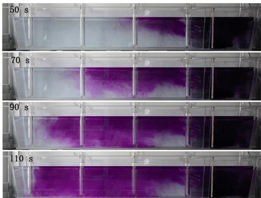
**Fig. 5** Flow field of prototype tundish
