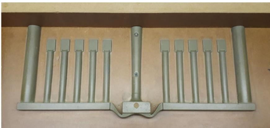
**Fig. 3** Photograph of the pattern used to obtain tensile test bars, with a well-designed running system, minimising the entrainment of double oxide film defects
