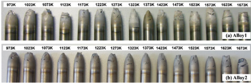
Fig. 6 Morphologies of fractures for the two alloys after tensile test
