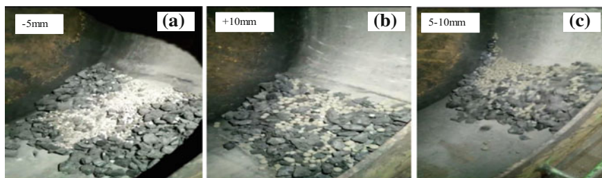
Fig. 6 The model of the segregation between coal and pellets
