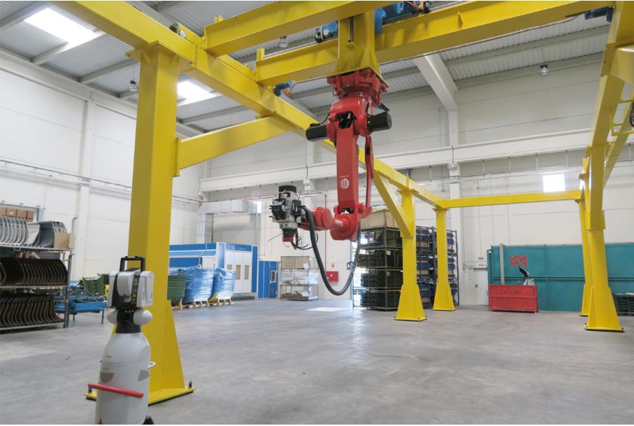
Fig. 1. Prototype system with CSEM control and Leica tracking system (installation at AITIIP, Zaragoza, Spain).
