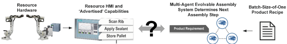
Fig. 2. A legacy production resource can be considered to be advertising its capabilities via a user interface. A smart manufacturing system such as an Evolvable Assembly System wishes to instantiate these capabilities. But how can the intelligent agents actually interface with the resource?
