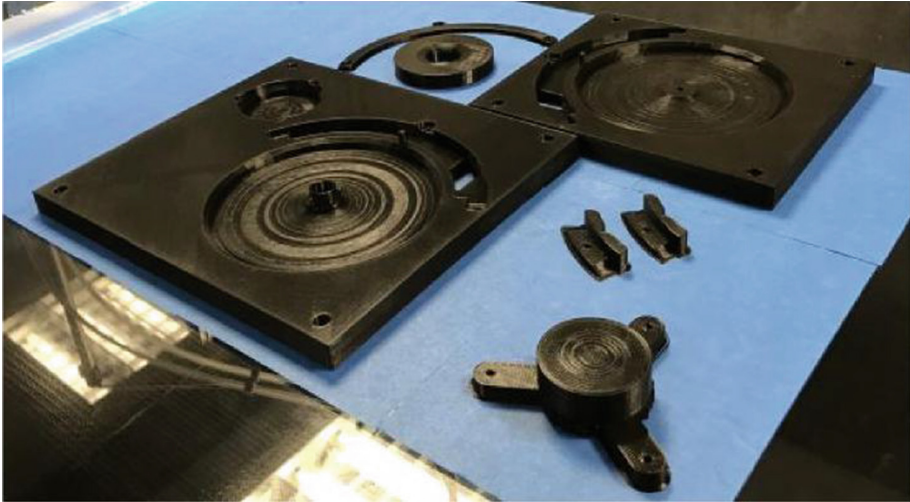
Fig. 8. An example of 3D printed parts used as fixture nests in a TQC machine
