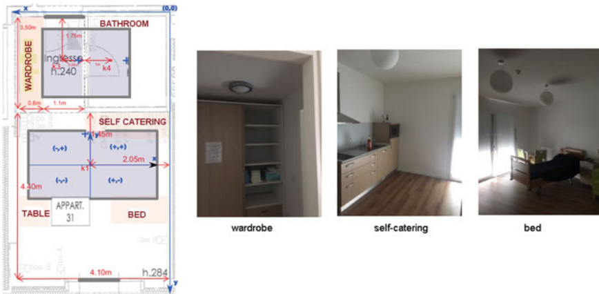
Fig. 4 Plan of the apartment where the pilot has been deployed. The entrance and the window are evidenced. The gray-shaded areas are those covered by the kinect sensors: one is located at the entrance in front of the wardrobe, the second is centered between the table, the self-catering and the bed. Details about the wardrobe, the self-catering and the bed positions are given in the corresponding pictures
