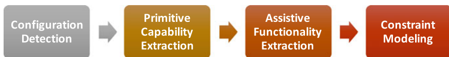
Fig. 3 Configuration pipeline for the generation of a timeline-based planning and acting model
