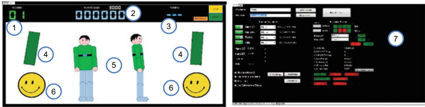
Fig. 3 Pictures of the user interface of PRESO software. (1) Round number of the exercise (if organized in rounds). (2) Score (in blue) and high-score (in white). (3) Countdown time in seconds, for the timed exercises. (4) Rectangles representing the inclination of the inertial sensors placed on the back of the hands. (5) Puppets reporting trunk’s inclination measured by the chest’s inertial module. (6) Smiles to give a nicer feedback about the inclination of the hands (smiling when in correct position, red and disappointed when not upright). (7) Parameter setup window, used by the therapist to check the information received from the sensors and to adjust the exercise parameter and select the exercises
