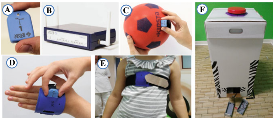
Fig. 1 A A Wavetrack sensing unit. B Wavetrack receiver. C Setup of the IMU sensor in the ball. D Placement of the IMU sensor in custom pocket on the back of the hand. E Positioning of the IMU sensor in a belt attached to the chest of the subject. F Plastic enclosure to hold a Cometa footswitch device to monitor the state of a big button (on the top of the cardboard box)
