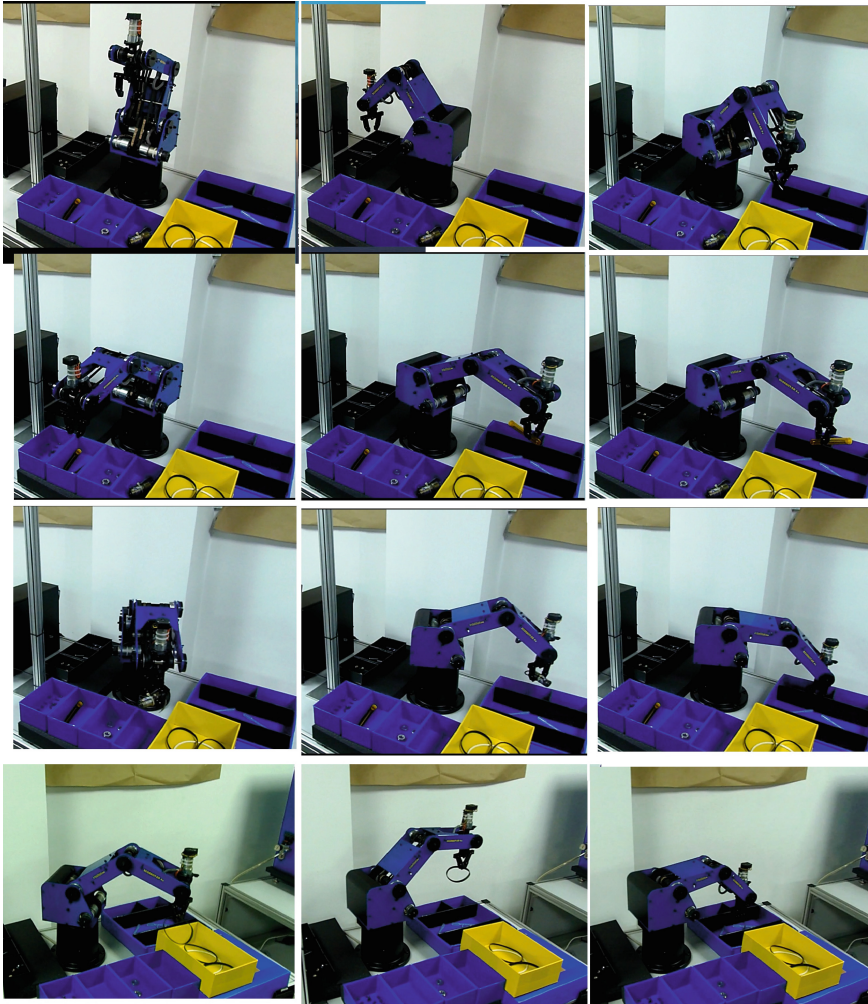
Fig. 6. Snapshots of intelligent picking from user inquiry, for different type of pieces, in order to achieve the kitting task. (Robot: Scorbot ER 4u)
