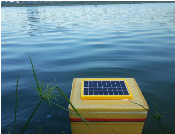
Fig. 16. (Live implementation of smart IoUT 1.0) operational in lake in Da Nang City capturing live water properties
