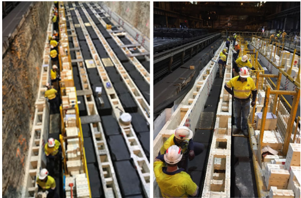
Fig. 10 Anode loading pattern in the BBA furnace with current and NG Technology
