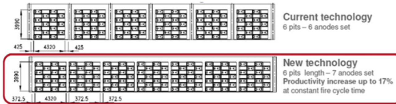
Fig. 10 Anode loading pattern in the BBA furnace with current and NG Technology
