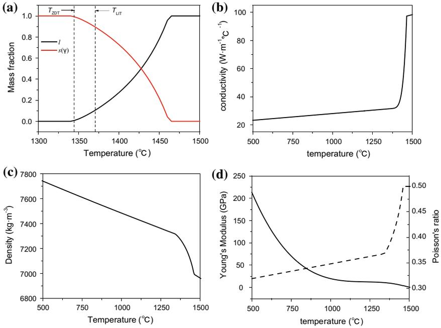
**Fig. 1** Phase fraction and material properties of C92 steel: **a** phase fraction, **b** conductivity, **c** density, **d** Young's modulus and Poisson's ratio
