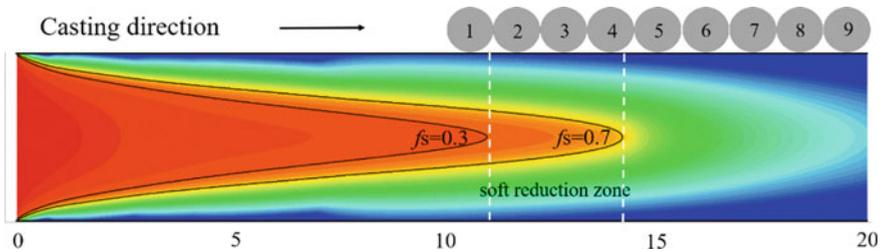
Fig. 3 Temperature distribution on longitudinal section of the bloom
