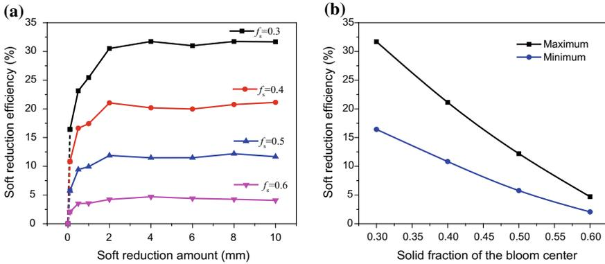
Fig. 7 Soft reduction efficiency of the bloom with convex rolls
