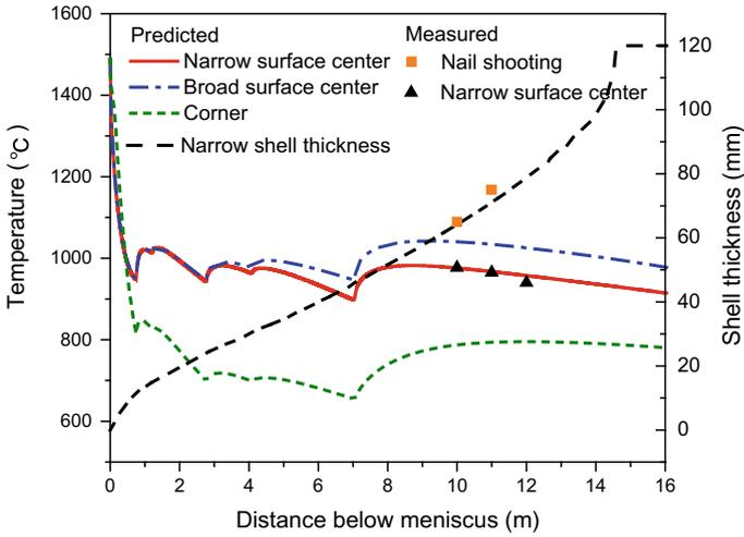
Fig. 2 Comparison between the predicted and measured surface temperature and shell thickness
