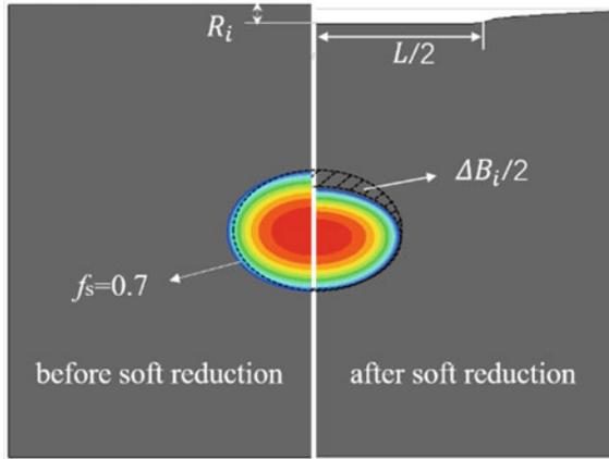
Fig. 6 Schematic of the CRSR process for bloom
