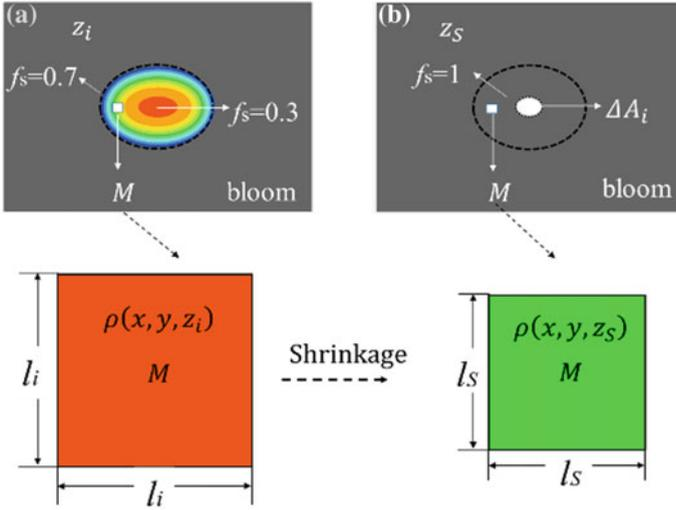
**Fig. 4** Schematic to calculate the solidification shrinkage of mushy zone
