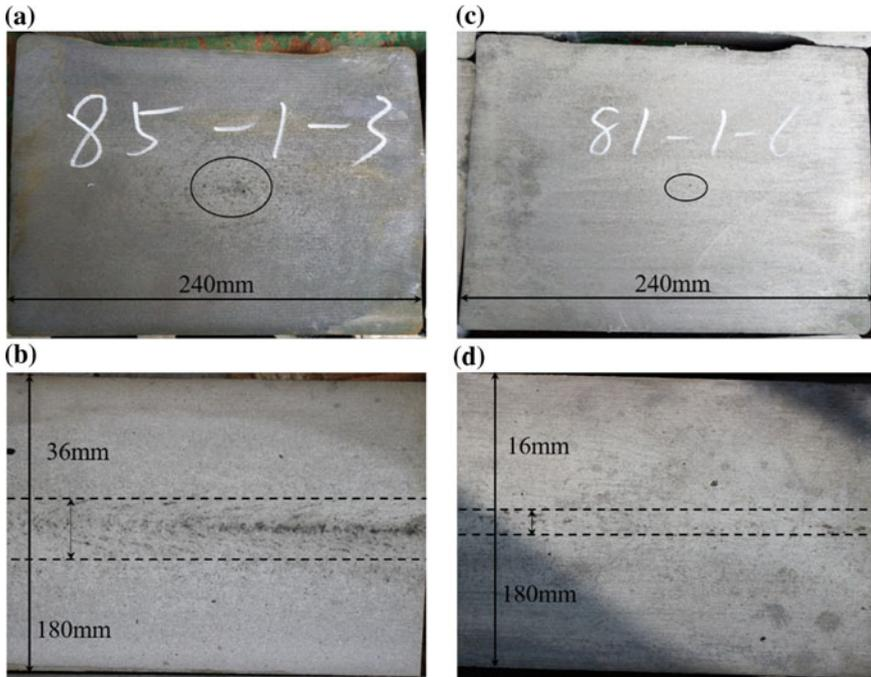
**Fig. 10** Macrographs of transverse (a, c) and longitudinal (b, d) bloom section: a and b old soft reduction amount, c and d optimum soft reduction amount calculated by model
