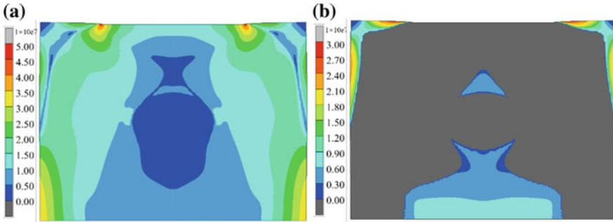
**Fig. 8** Stress distribution of the bloom during the soft reduction with convex rolls ( $f_s = 0.3$ , SR amount = 2 mm): **a** equivalent of stress, **b** major principle tensile stress (unit: Pa)
