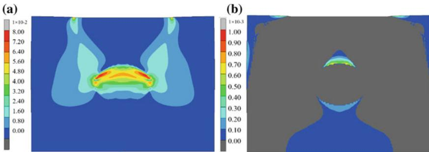
**Fig. 9** Strain distribution of the bloom during the soft reduction with convex rolls ( $f_s = 0.3$ , SR amount = 2 mm): **a** equivalent of plastic strain, **b** major principle tensile plastic strain
