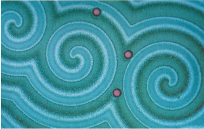
Fig. 7 Counter-rotating spirals in the BZ reaction, visualized in pseudo-color. Each of these spirals have an almost Archimedean shape and their tips rotate uniformly around a spatially fixed center. Note that wave fronts mutually annihilate each other upon collision. (Circular inclusions are CO 2 bubbles.) Reprint from [6], permission obtained from Springer Basel AG
