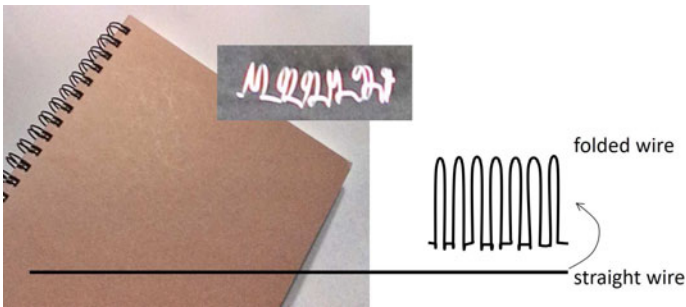
Fig. 10 A ring book and its wiring, insert: wire removed from the ring book. A long wire is folded as shown in the right drawing
