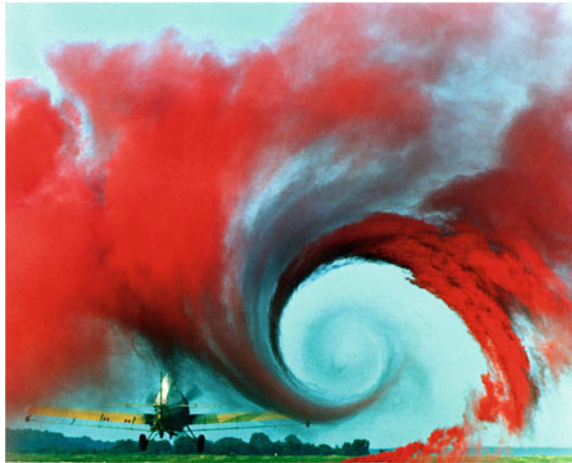
Fig. 8 Wake turbulence of large aircraft. The air flow from the wing of the plane was made visible by using colored smoke rising from the ground. Photographed by NASA langley research center (NASA-LaRC)
