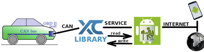
Fig. 1. A schematic description of the connection between car and OpenXC.
