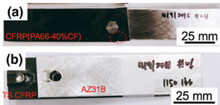
Fig. 6 a Fractography of thermoplastic CFRP (PA66-40%CF) joined to AZ31B by friction self-piercing riveting, showing net tension failure of the composite (red-dotted circle). b Fractography of thermoset CFRP (G-83 prepreg) joined to AZ31B showing pullout from the AZ31B
