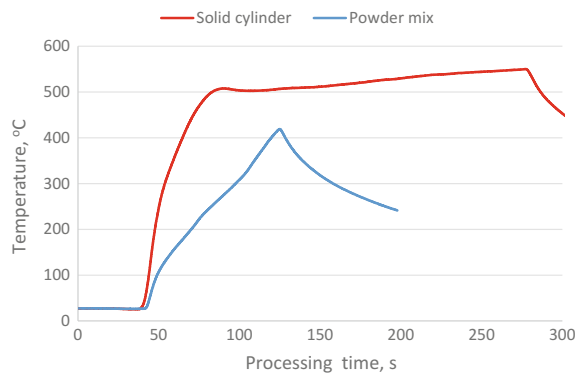
Fig. 6 Die face temperature during ShAPE process
