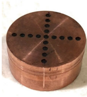
Fig. 1 Copper disc with pre-drilled holes
