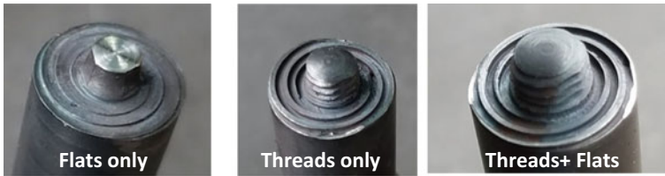
Fig. 2 Representative FSLW tools with different shoulder and pin features
