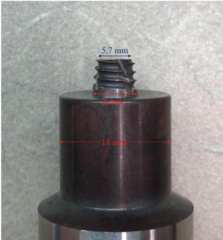
Fig. 1 D10314A monolithic friction stir tool made of H13 tool steel by Bond Technologies
