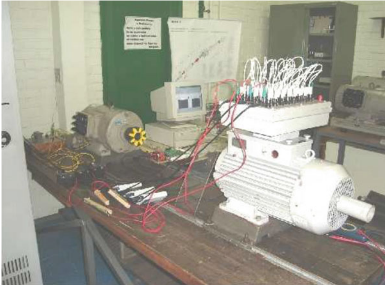
Fig. 9 Instrumental setup and motor external connections
