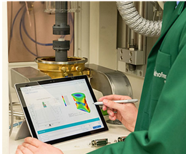
Fig. 12 Process monitoring during precision glass molding [32]
