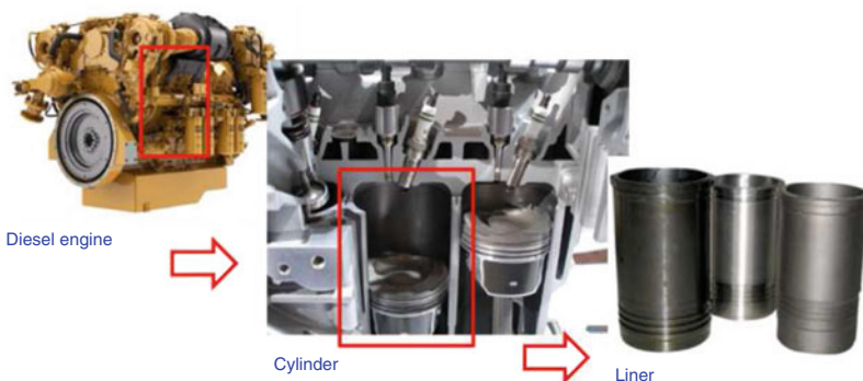
Fig. 12 Position of cylinder liner and piston rings in a diesel engine
