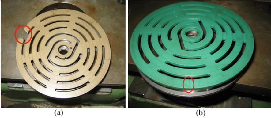
Fig. 22 Faulty sealing elements of a plate valve. (a) The sealing element of a plate valve with a part broken off (fault state = Broken ). (b) The sealing element of a plate valve with a fissure (fault state = Crack )
