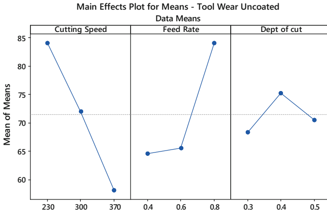
Fig. 4 Main effect plot for means of tool wear
