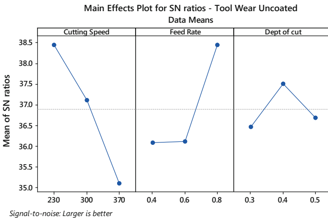
Fig. 3 Main effect plot for S/N ratios of tool wear
