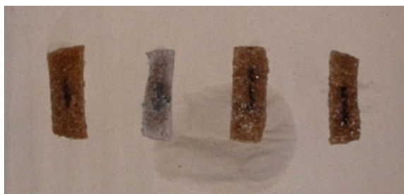
Fig. 9 Effect of Sulphur acid in swamp water changes colour from brown to white
