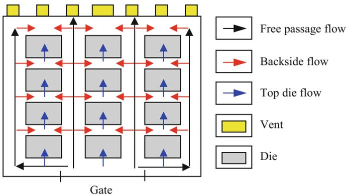
Fig. 3 Schematic of flow in the cavity
