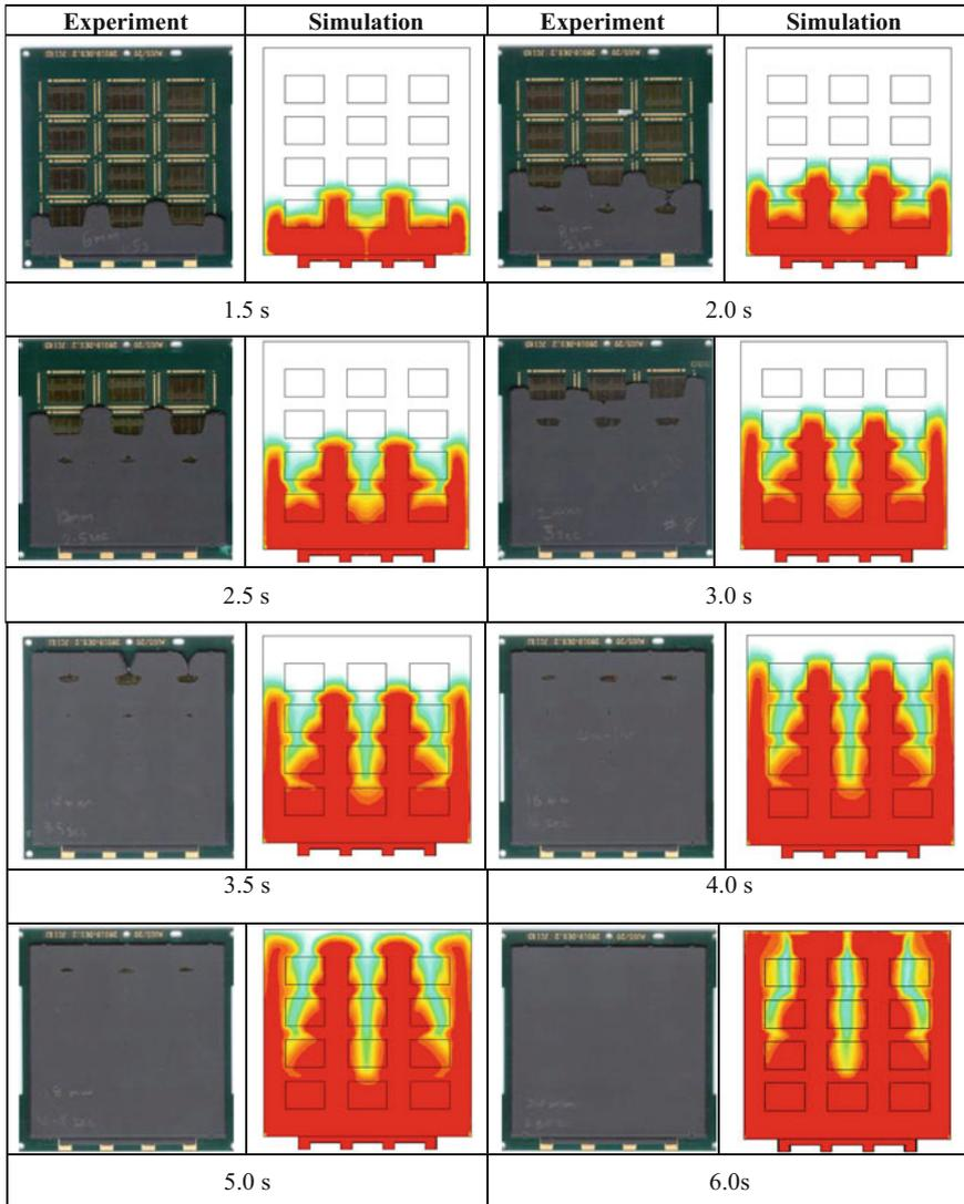
**Fig. 4** Short shot results of melt front advancement at distinct time steps with velocity inlet of 4 mm/s
