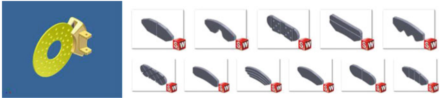
Fig. 4 Brake pads part design using solidworks
