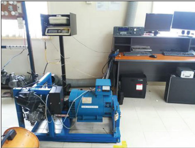
Fig. 1 Experimental setup for gasoline engine performance measurement
