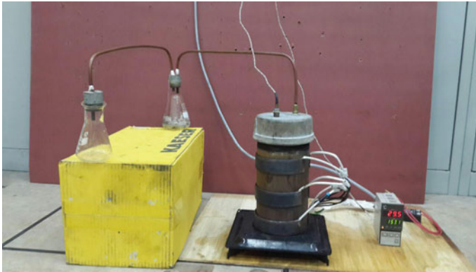
Fig. 4 Experimental setup of the pyrolysis process
