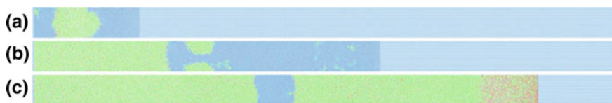
Fig. 8.2 MD snapshots of a shock to detonation transition in a model AB explosive with a 5 nm radius void shocked at U_p = 4 km/s. Shock travels from left to right. Blue atoms denote unreacted material, green atoms represent product molecules while red atoms are unbonded monoatomic species. Snapshots show a Collapse of a void and the formation of a deflagration wave, b formation of hotspots between the deflagration wave and the shock front that ultimately give rise to a detonation (c) . Reproduced with permission from [45]. Copyright (2010), American Physical Society
