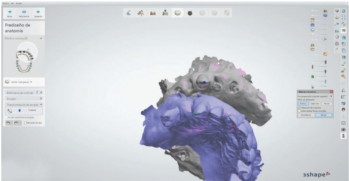
Fig. 19 Merging (best fit) of study model (consultation, preoperative) scan (blue) and implant file. Marking same points on both scans allow the software to import the study model scan as a pre-preparation on the final working file
