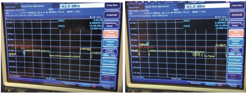
Fig. 5. The traffic injected by the BS on channel 2 under default (left hand side) and optimal (right hand side) transmission burst length settings.
